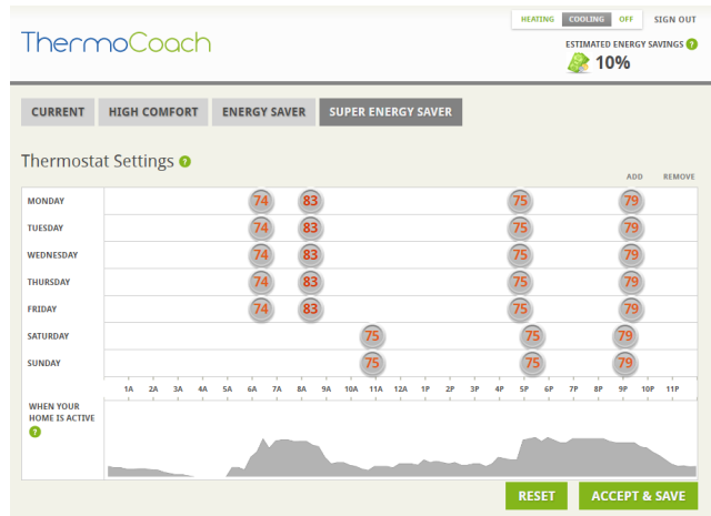
Figure 2. ThermoCoach web page allows users to view and edit detailed thermostat schedule options. Users can select a schedule option from menu (top left). While editing, users are informed of estimated energy savings (top right) based on the current settings. The graph along the bottom shows the times when their home is typically active.
