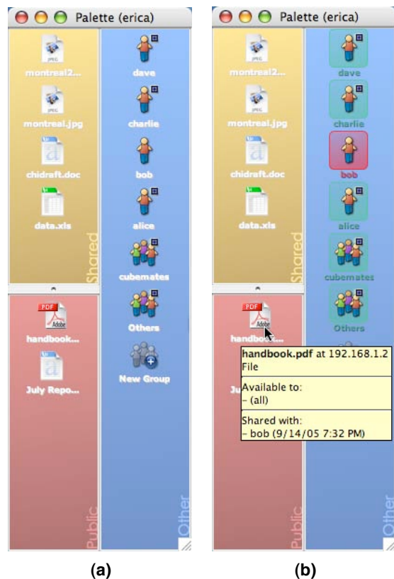
Figure 1: (a) A prototype of the sharing palette user interface. (b) Using the sharing palette to discover with whom the file handbook.pdf is currently shared.
